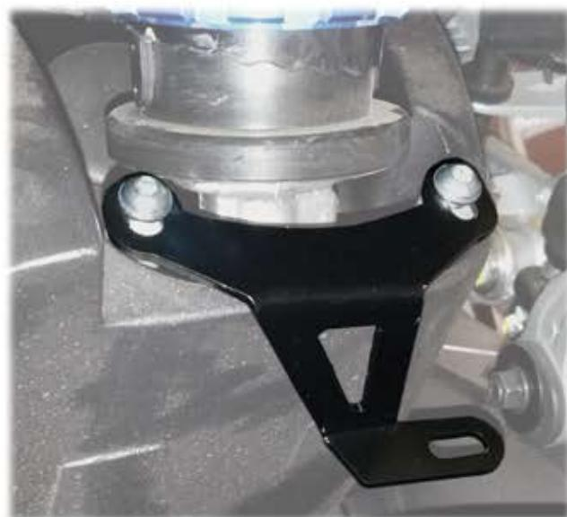
REMOVE THE ORIGINAL CHAIN COVER FROM THE MOTORBIKE AND THE TWO SCREWS FROM THE REAR SHOCK ABSORBER. USE THE TWO THICKNESS TO FIX THE BRACKET LIKE DESCRIBED IN THE PICTURE. ONCE FIXED THE BRACKET WE ADVICE TO SEPARATE THE ABS PART FROM THE ALUMINIUM CHAIN COVER SO YOU CAN FIX ON THE MOTORBIKE.
